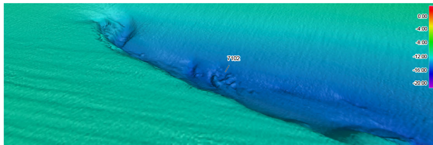
Multibeam bathymetry image of seabed disturbance 7102, looking north, x1 vertical exaggeration
